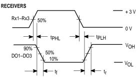
Figure 2. Switching Characteristics
