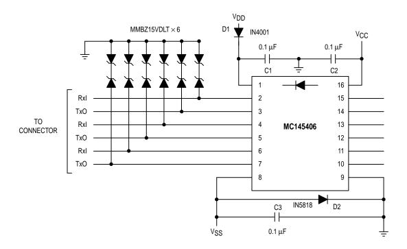
Figure 4. ESD and Power Supply Networks
