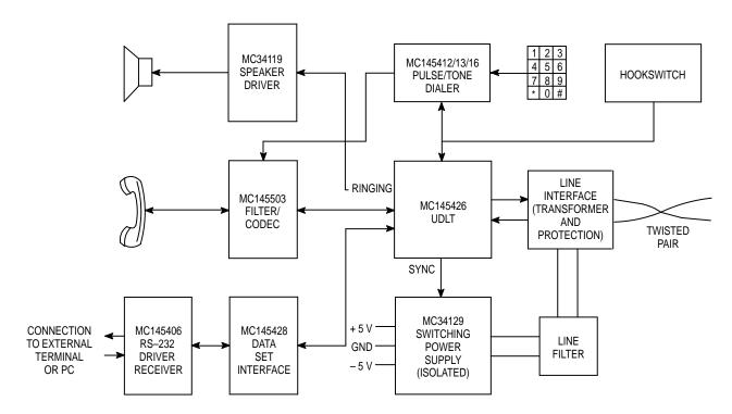
Figure 6. Line-Powered Voice/Data Telephone with Electrically Isolated EIA 232-E Interface
