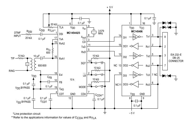
Figure 5. 5-V 300-Baud Modem with EIA 232-E Interface
